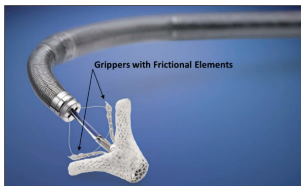
Figure 4. The first-generation MitraClip™ device with grippers and FEs distributed along the length of the grippers, which prevents the leaflets from slipping out of the Clip arms during Clip closure and maintains the Clip's long-term attachment to both MV leaflets.
